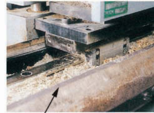
Running test in wood chips
