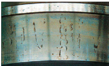
Rust and corrosion
