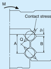
Fig. 2 Enlarged illustration: Offset Gothic arch
