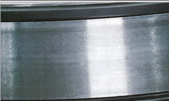
DENTING: Indentation, surface depressions in a metal surface
