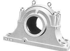
These types are large and made for heavy loads. Standard models have double seals and four mounting bolt holes. Types SD2C and SD3C feature different bore diameters on both sides.
