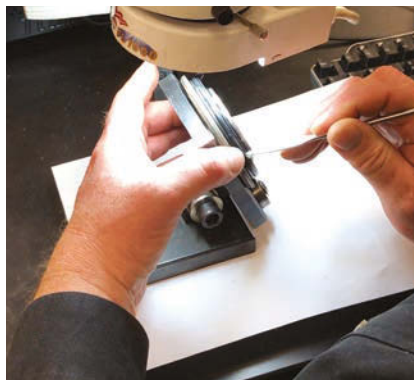
Grease samples were taken from seal lips for analysis.
