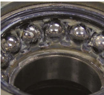
Ample amount of clean grease on bearing balls and cage - no dirt or grease contamination.
