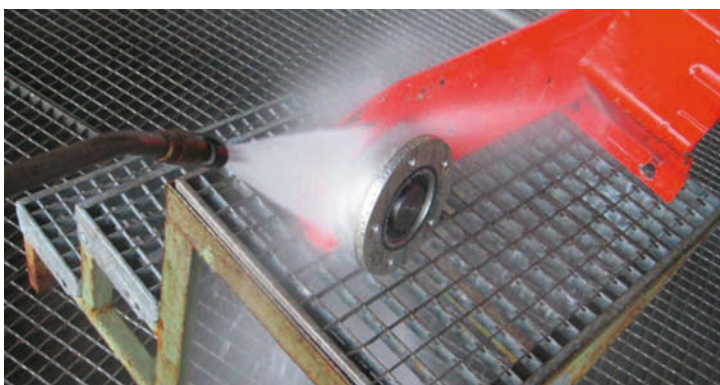
Figure 3: Tested using a water jet for 200 hours. At the end of the test, there was no sign of water having penetrated the cassette seal.
