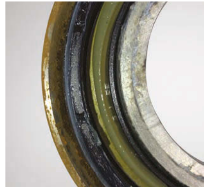
Clean grease on cartridge seal - no signs of dirt past 2nd lip seal.
