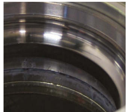
Raceways are in like-new condition.
