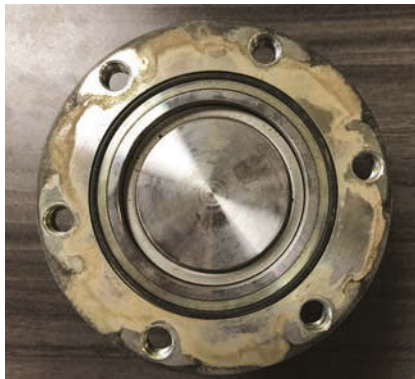
NSK hub flange side with O-ring seal.
