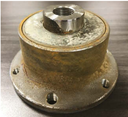
NSK Agri hub after over 4,500 acres of use - no external damage.
