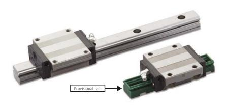
For interchangeable NH and NS Series linear guides, the ball slides and the rails are stocked separately. The ball slides are mounted on plastic provisional rails that allows for easy transfer of the ball slide to and from the steel rail.
