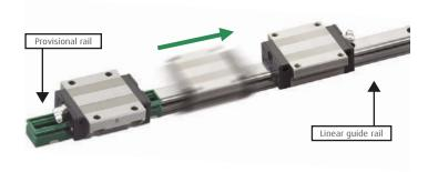
If a ball is accidentally dropped from the ball slide, it should be cleaned and replaced to the appropriate groove. The correct groove can be determined by the size of the clearance between the balls (the groove missing the ball will have greater clearance than the other grooves). It is normal to have a gap of 1.5 ball diameters in each groove.
