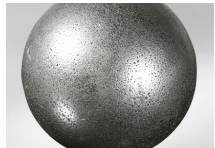
Part: Ball of Photo 6.9.1 Observation: Pitting occurs on the rolling element surface
