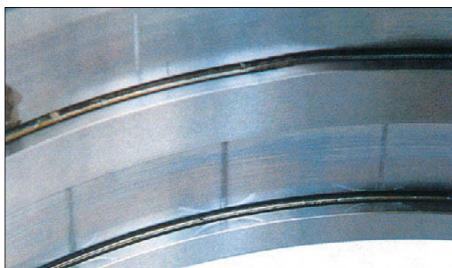
Part: Outer ring of a double-row cylindrical roller bearing Symptom: Fretting occurs on the raceway surface at roller pitch intervals
