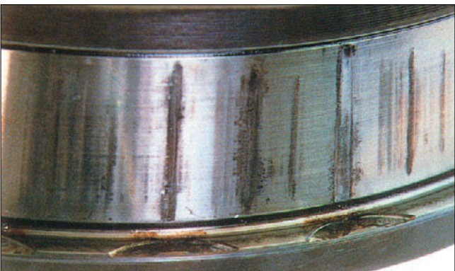
Part: Inner ring of a double-row tapered roller bearing Symptom: Fretting wear of raceway and stepped wear on the rib face Cause: Fretting progression due to excessive load while stationary
