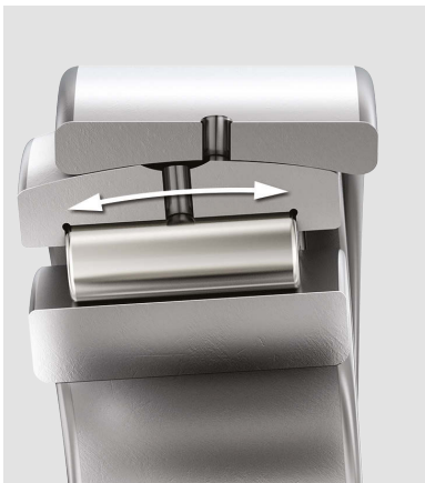
Aligning ring tolerates misalignment and shaft deflection
