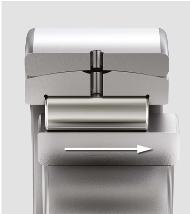
Smooth axial displacement accommodates free thermal expansion of the roll
