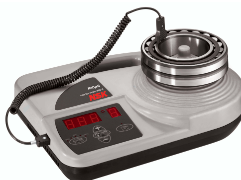
Fig. 5: Heating by bearing heater
