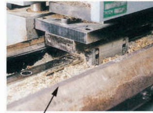
Running test in wood chips
