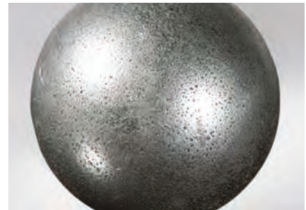
Part: Ball of Photo 9.1 Observation: Pitting occurs on the rolling element surface
