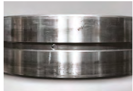
Part: Outer ring of a spherical roller bearing Observation: Creep occurs over entire circumference of outside surface Cause: Loose fit between outer ring and housing
