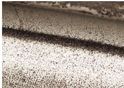
Part: Outer ring of a slewing bearing Observation: Pitting occurs on the raceway surface Cause: Rust at bottoms of indentations
