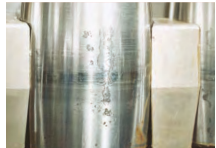
Part: Rollers of a spherical roller bearing Observation: Pit-shaped rust on rolling contact surface; corroded portions Cause: Moisture condensation during storage
