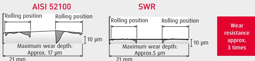
Evaluation of an endurance test using 22210CD bearings
