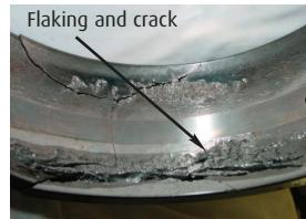
Outer ring raceway surface
