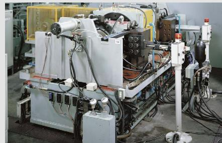
Test rig for bearings used in work rolls
