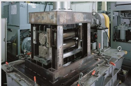
Test rig for bearings used in guide rolls
