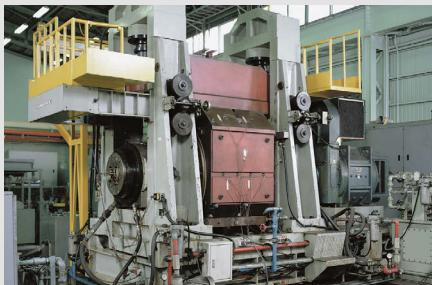
Test rig for bearings used in backup rolls
