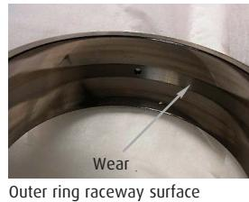
Outer ring raceway surface
